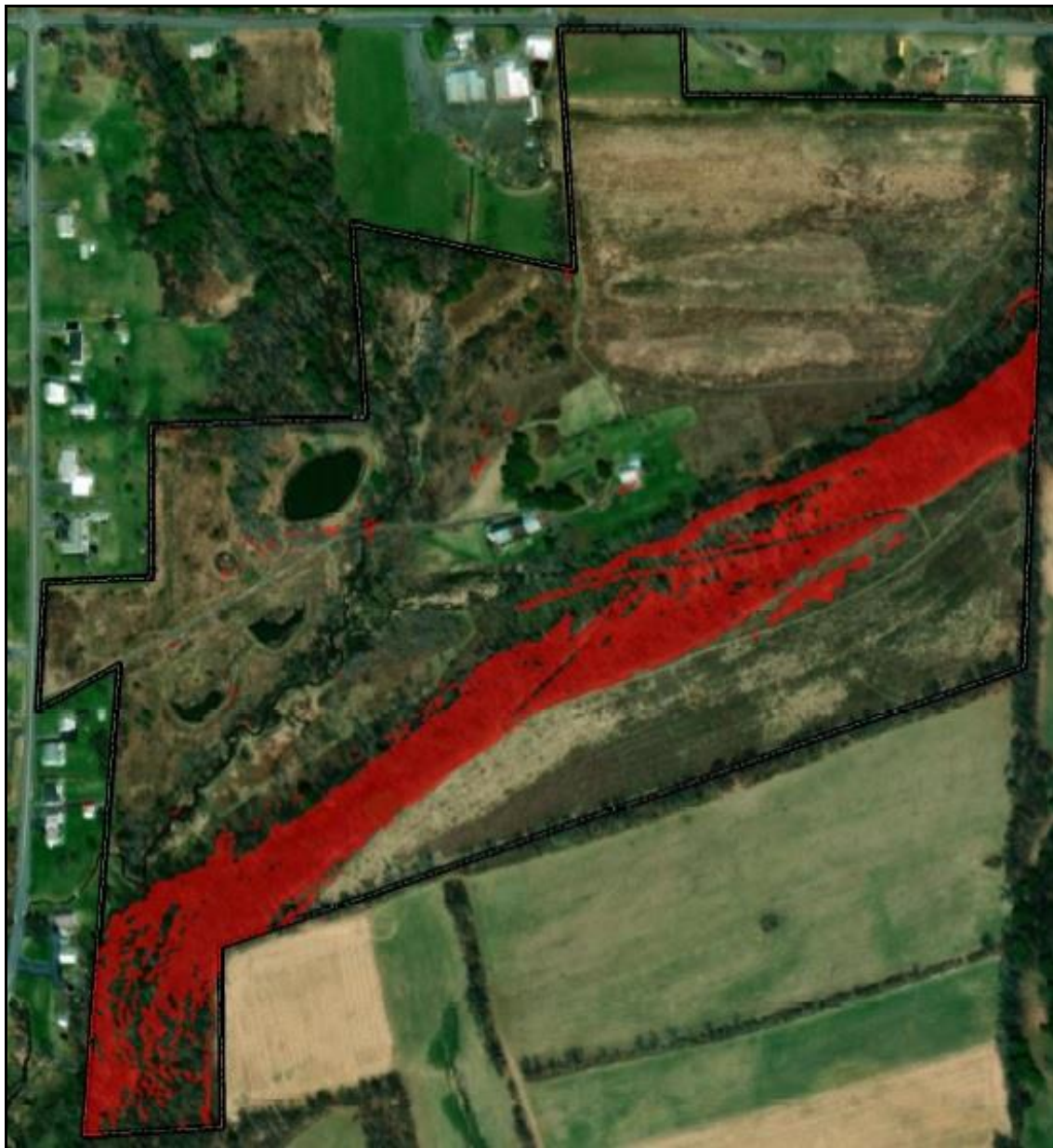
Red Band indicates slope in excess of 40% as generated by digital elevation model analysis (Green Leaf Consulting Services, LLC.)
